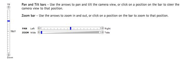
The PTZ controls can be disabled under PTZ > Advanced > Controls, see Controls, on page 23.
